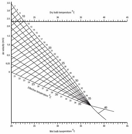
Wet bulb temperature would be lower than dry bulb when the air is not saturated with water vapour. Body temperature is 37°C. The graph takes a bit of getting used to.
